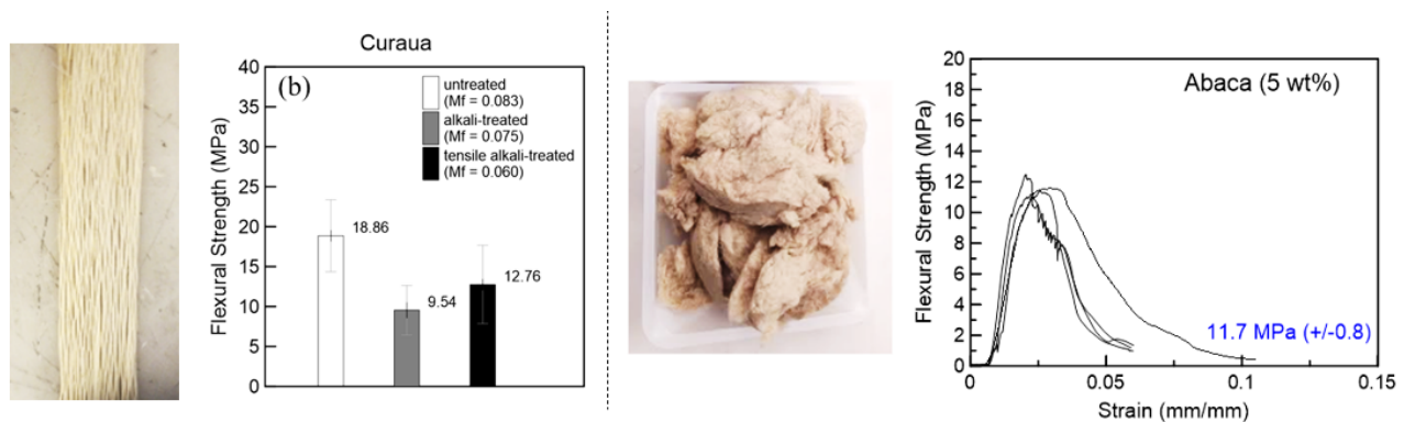
Figure 1 – Curaua and Abaca fiber arrangements, and the composites flexural strengths.
