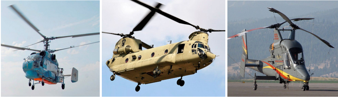
Figure 1.1: Coaxial Kamov [9], Counter-Rotating Chinook [10], and Intermeshing-Rotor Kaman [11] Helicopters
