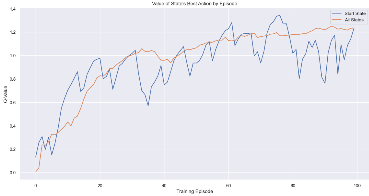
Figure 7.4 Average Q-Values for all trained state-action pairs and the initial AISOSVM model states.
