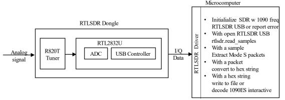
The core of the RTL2832U transponder is an analogue-to-digital converter that samples the radio waves and digitizes those samples (Laufer, 2014; Lichtman, 2023). The USB controller on the RTL2832U then makes the resulting I/Q data, In-Phase and Quadrature, available to the software driver on the microcomputer. The I/Q data is processed into Mode S messages.
