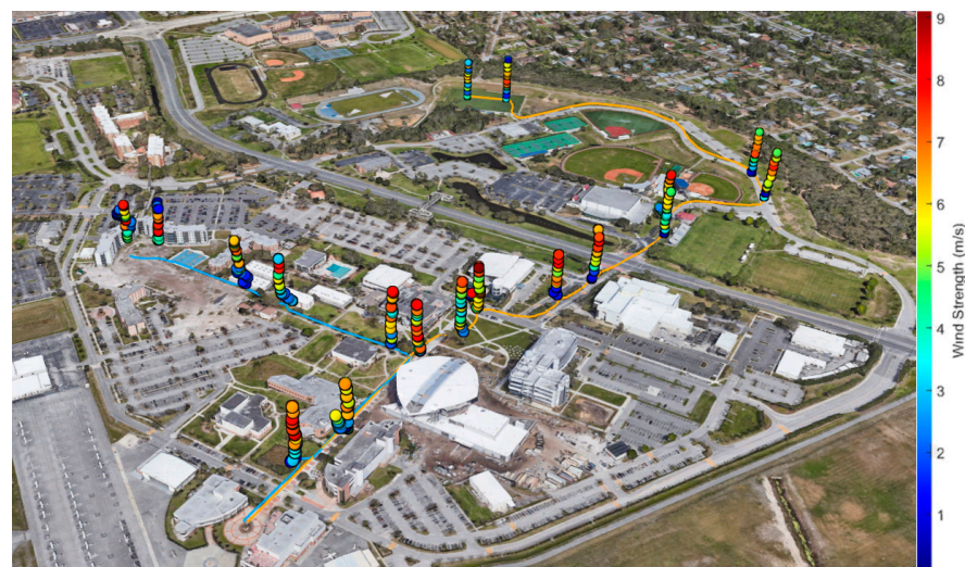
Figure 13. Vertically stacked observations taken along the urban route (blue) and suburban route (orange). Image courtesy of Google Earth. However, image shown is not up to date at the time when the field validation was undertaken. Mid-rise buildings and urban canyons are not reflected in this image.
