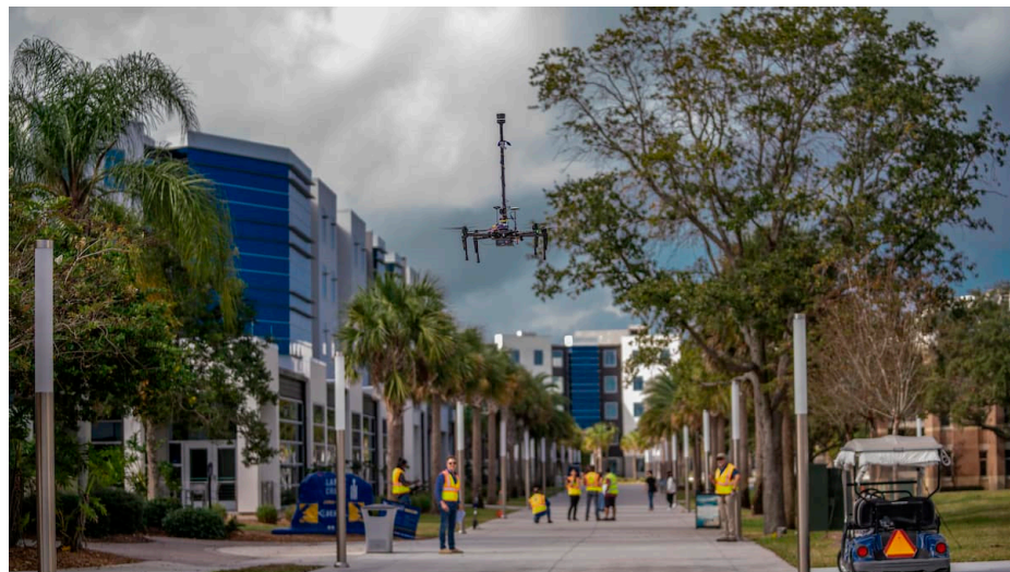
Figure 11. A meteorologically instrumented uncrewed aircraft participating in the GUMP field campaign.
