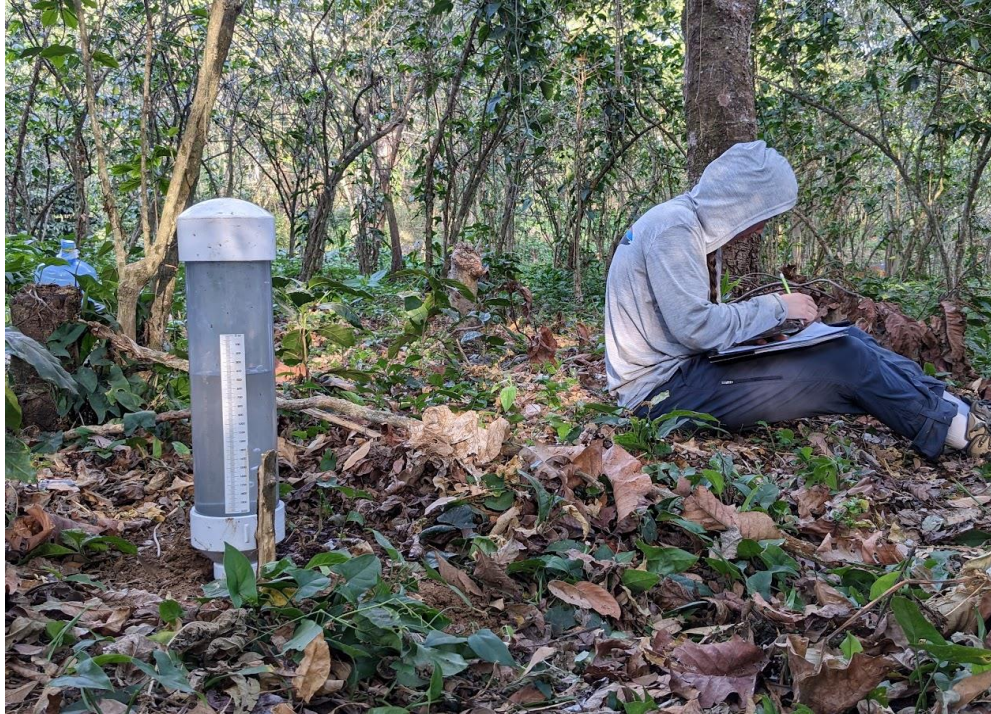
Figure 19: Conducting infiltrrometer tests in the field using the Perm-It™ constant-head infiltrrometer.
