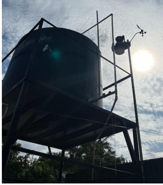
Figure 8: Installed Vantage Pro2™ weather station.
