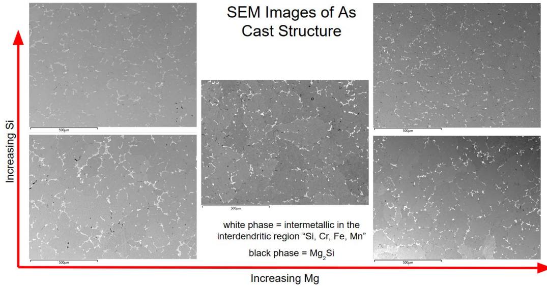
Figure 21. BSE images of the as-cast structure with increasing Mg and Si. The black is the Mg_2Si phase, and the white is the intermetallic in the interdendritic microconstituent.
