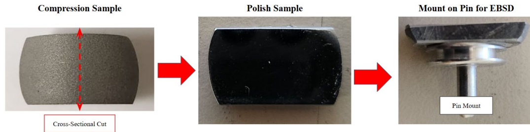
Figure 18. EBSD sample preparation from compressed sample
