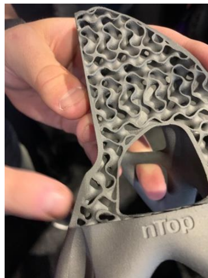
Figure 12. NASA Excite Challenge Bracket showing the variations in the lattice wall thickness within the part.
