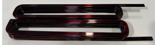
Fig 1. Typical coil windings formed from edgewise enamelled wires.
