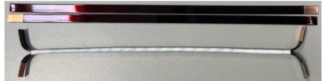
Fig. 2. Edgewise insulated wires (top) before and (below) after wrapping in PTFE, test sample.
