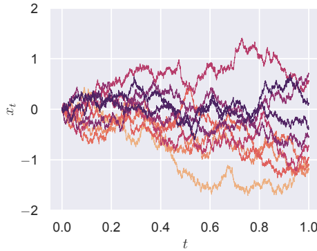
Figure 3.1: Illustration of the Girsanov theorem in action. The plotted paths were sampled from the Wiener measure, and colored according to the Radon-Nikodym derivative of the measure induced by the OU process dX_t = -X_t dt + dW_t against the Wiener measure. Since the OU process reverts to 0, paths that deviate farther from 0 have lower RND.
