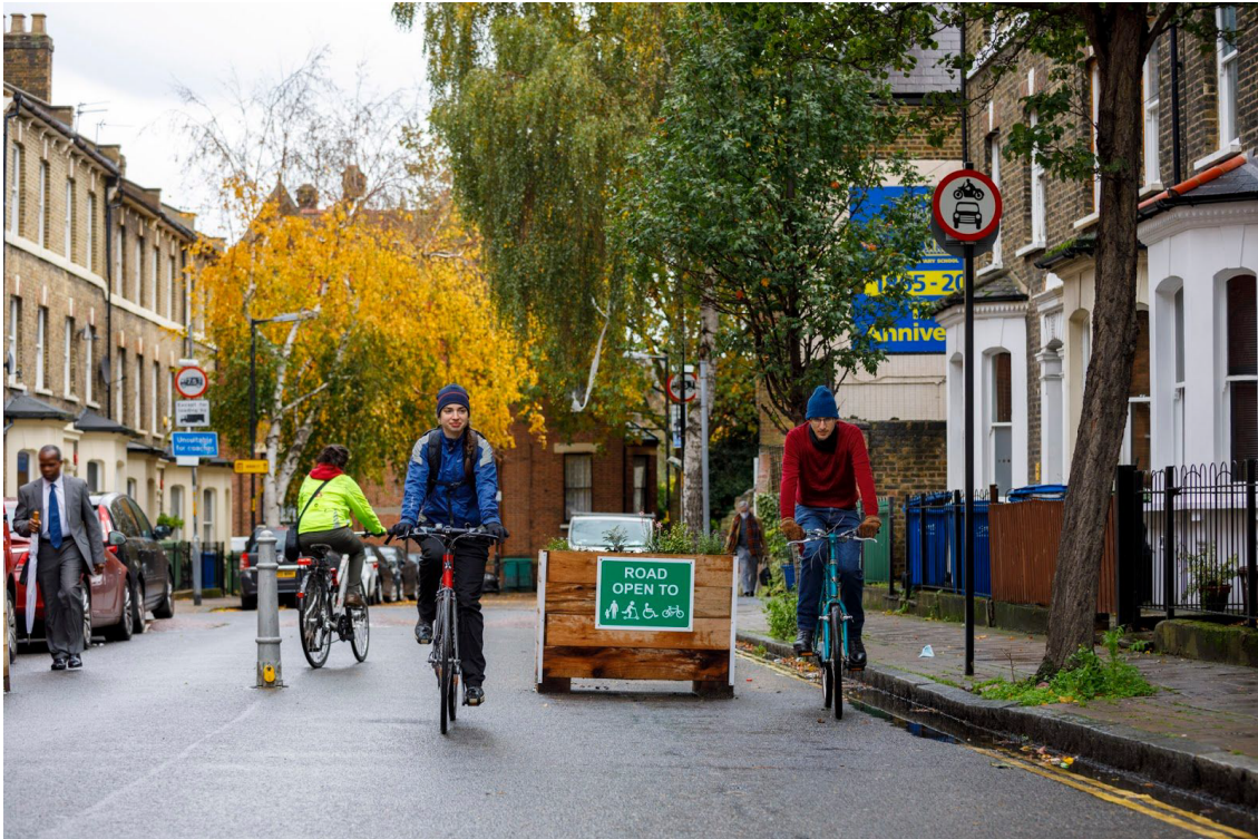
Figure 2. A typical modal filter used to stop cars and allow walking, wheeling and cycling (image credit: Crispin Hughes)
