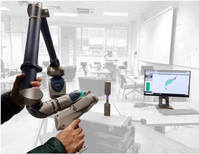
Fig. 5. Laser scanning of a typical fatigue coupon.
