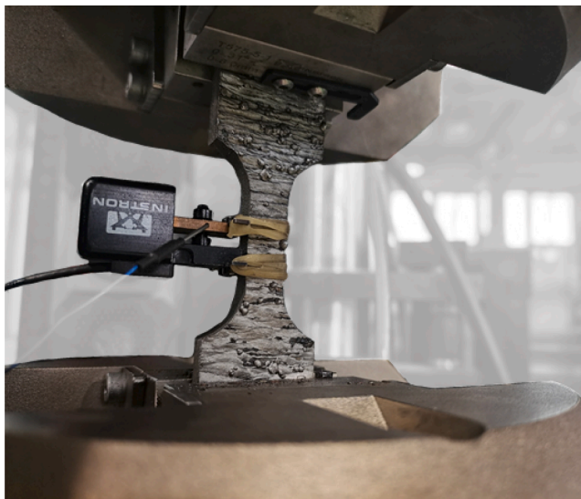
Fig. 7. Setup for axial LCF tests.
