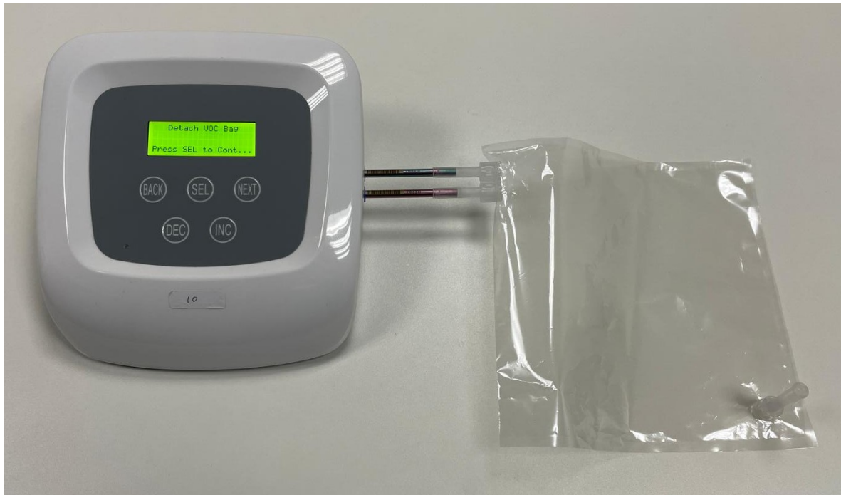
Figure 3.8 Photograph of novel breath collection device connected to two TD tubes and the final design of PTFE breath sampling bag.
