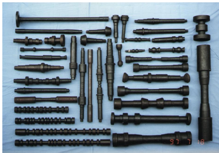
Figure 1.2 Various cross wedge rolling products [2].
