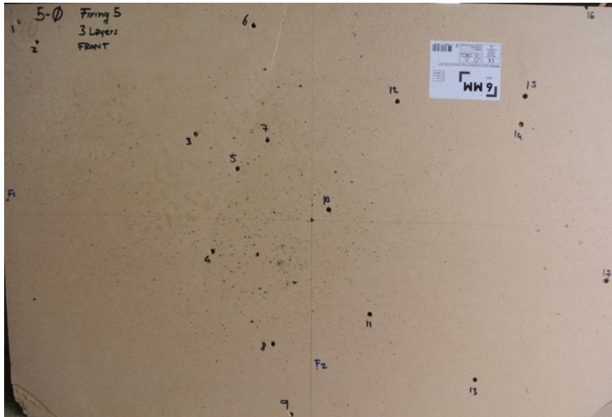
Figure 8 – 6 mm thick MDF front sheet post exposure to a 100 g charge of PE8 containing 75 ball bearings at 1 m range.
