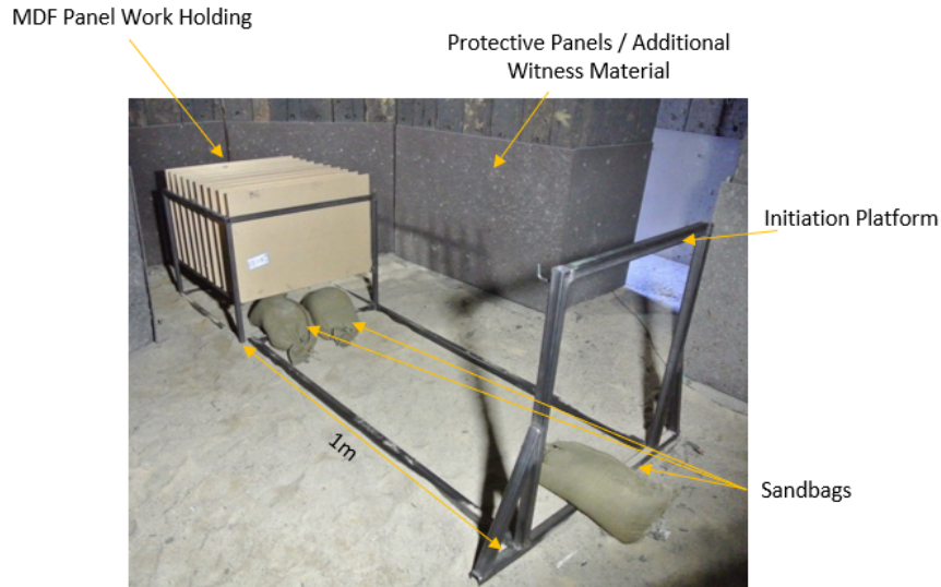
Figure 6 - Test Set Up / Rig Design
