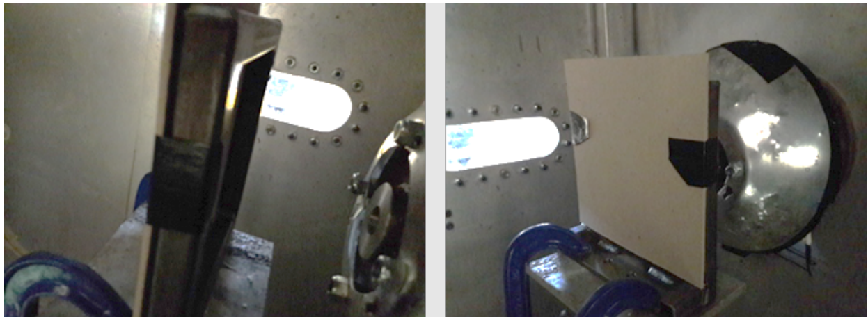
Figure 2 - Target Set Up within the ELVIS Gas Gun target chamber and view of Sabot Stripper
