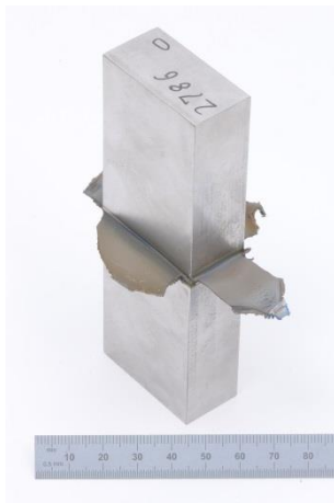
Weld 25 (note that there is also a noticeable HAZ)
