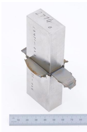
Weld 13 (note that there is also a noticeable HAZ)
