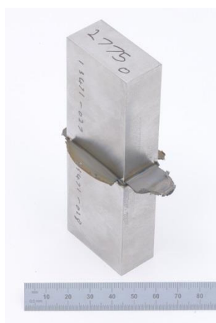
Weld 14 (note that there is also a noticeable HAZ)
