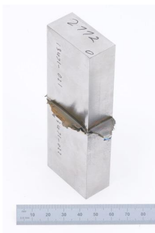
Weld 11 (note that there is also a noticeable HAZ – 2.9 mm)
