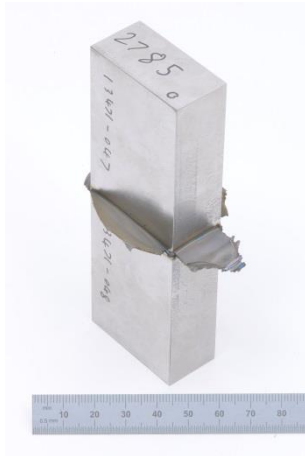
Weld 24 (note that there is also a noticeable HAZ)
