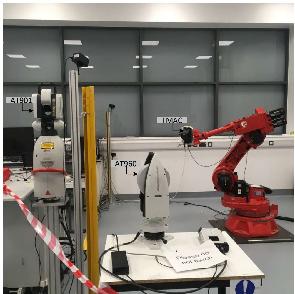
Figure 16. AT960 Leica Tracker Setup for NRTEC Verification.
