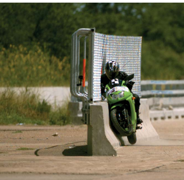
Similar crash tests have been done at TTI in the past, testing trajectory and interaction between the motorcycle rider and the net system during an impact event.
