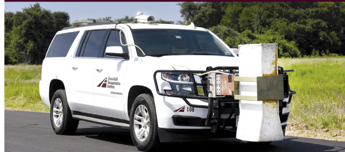
Air-coupled GPR transmits pulses of radar energy to collect data at highway speeds. Layer thicknesses and locations of air- and water-filled voids and layers with excess moisture or excess air voids can be determined using this device.
