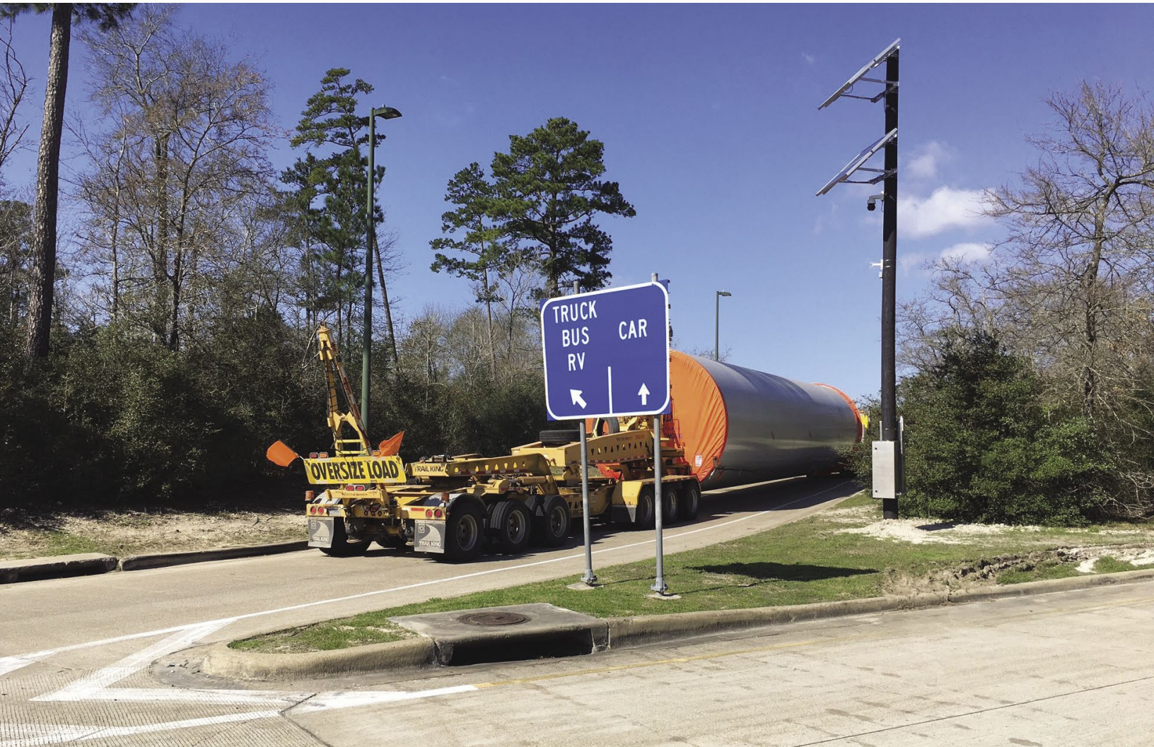
An oversized truck entering a northbound I-45 safety rest area. Notice the TTI-developed entry detection system located on the utility pole.
