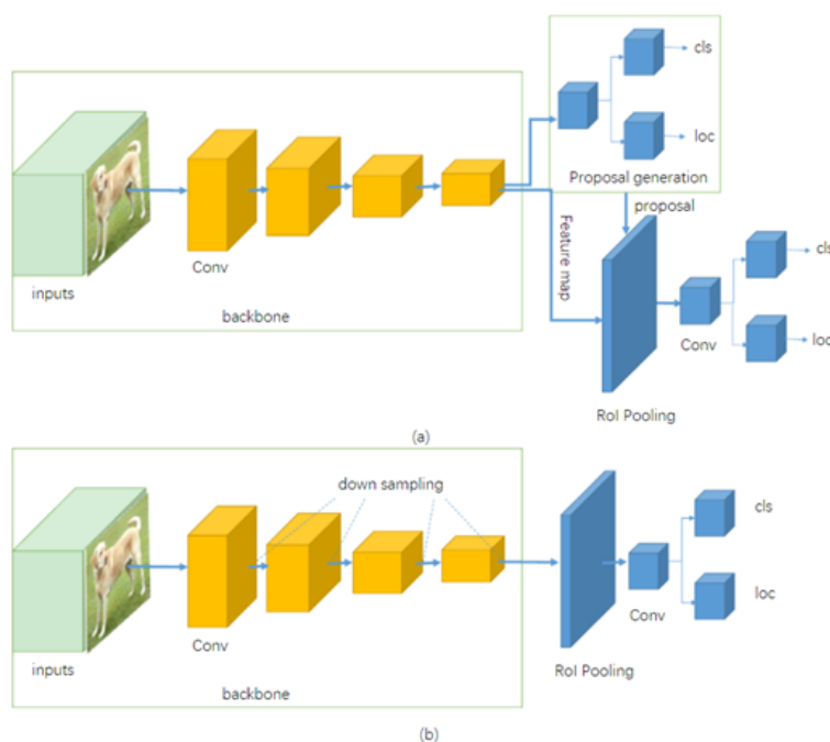
Figure 2. One-stage and two-stage Object Detection model architecture [18]
