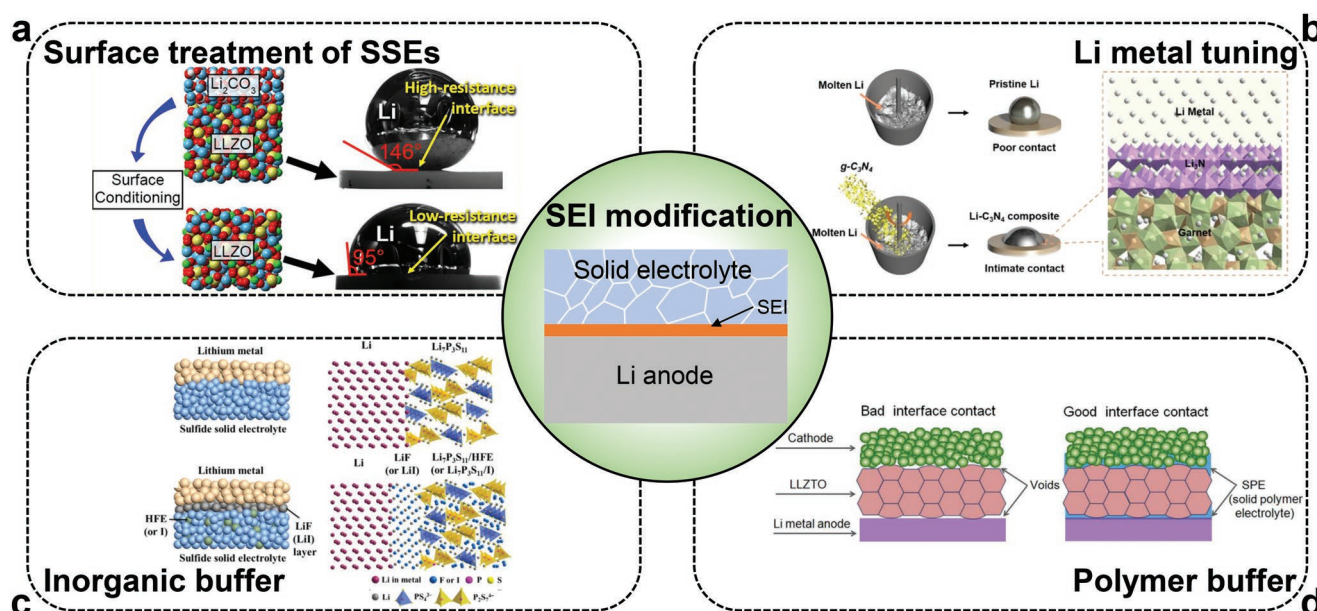
Figure 4. Schematic illustration of SEI modification strategies for Li anode in solid electrolytes. a) Surface of LLZO and contact angle of molten metallic Li before and after surface control. Reproduced with permission. [130] Copyright 2017, American Chemical Society. b) The synthesis process of Li-C_3N_4 composite and the interfacial contact comparison of Li/garnet and Li-C_3N_4/garnet . Reproduced with permission. [133] Copyright 2019, Royal Society of Chemistry. c) Schematic diagrams of Li/Li_7P_3S_{11} interface and modified interface with a uniform thin LiF (or LiI ) interphase layer and HFE (or I solution) infiltrated sulfide electrolyte. Reproduced with permission. [139] Copyright 2018, Elsevier. d) Schematic illustration of the conventional solid-state battery and solid polymer electrolyte layer-applied solid-state battery. Reproduced with permission. [147] Copyright 2019, Elsevier.
