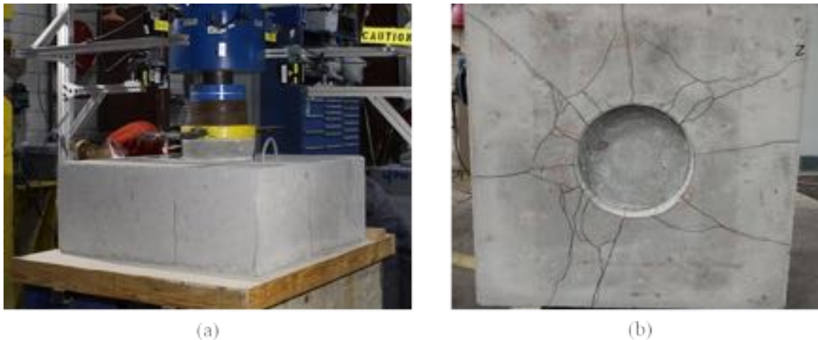
Figure A - 122: Specimen S3-1 (a) elevation during testing and (b) bottom cracking after testing. The stresses in the vertical reinforcement were also measured. As well as the confining reinforcement, the west side was more engaged than the north side of the specimen as shown in Figure A - 123. In addition, similar stresses were found in the cap and the plug
