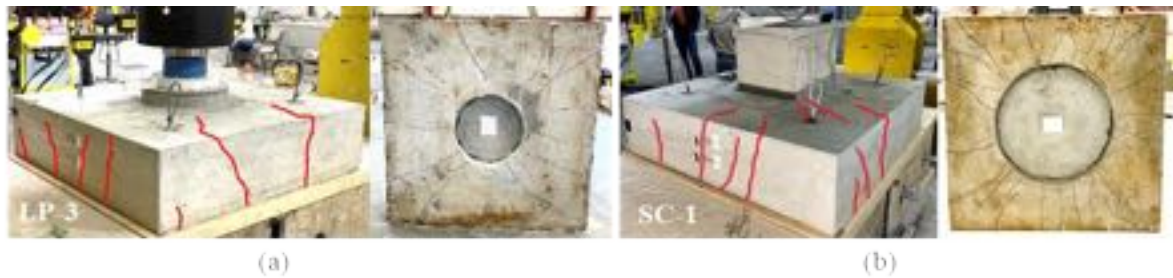
Figure 3-90: Crack patterns at failure for LP and SC specimens with corrugated interface (a) LP-3 and (b) SC-1
