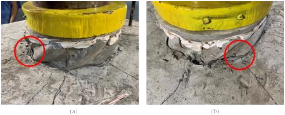
Figure A - 73: Details of plug rotation in (a) separation of the interface is observed and in (b) reference lines does not mach.
