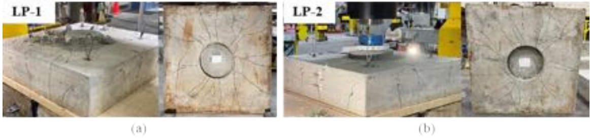
Figure 3-76: Crack patterns at failure for (a) LP-1 (1/16-inch roughness) and (b) LP-2 (1/4-inch roughness) without corrugations
