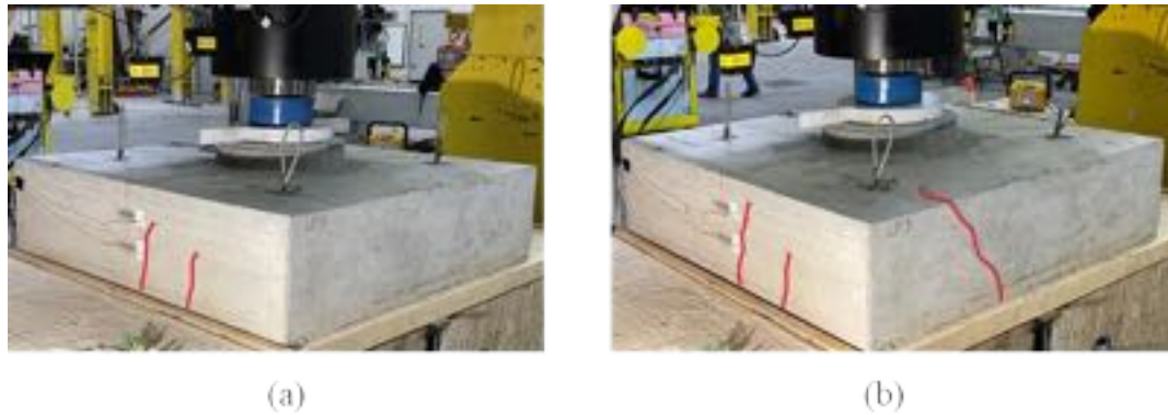
Figure B - 17: Crack progression for LP-3 during testing at (a) 200 kips and (b) 300 kips
