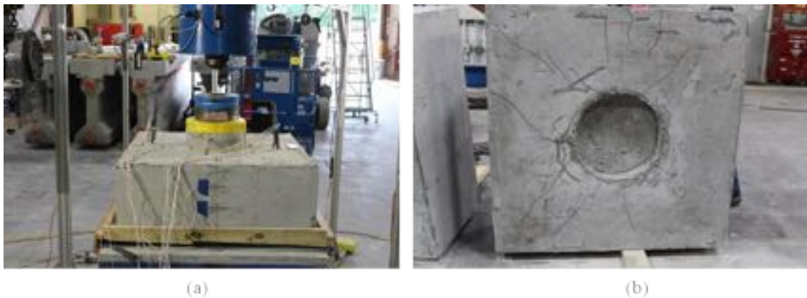
Figure A - 41: Specimen S2-4 (a) elevation before testing and (b) bottom cracking after testing
