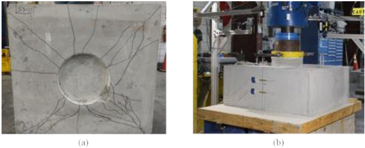
Figure A - 179: Cracking on (a) bottom after testing and (b) cap during testing of Specimen S3-11
