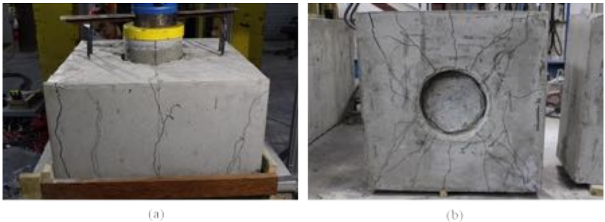
Figure A - 65: Cracking on (a) cap and (b) bottom of Specimen S2-8
