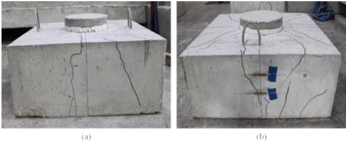
Figure A - 100: Cracking on the (a) south side and (b) east side on specimen S2-14
