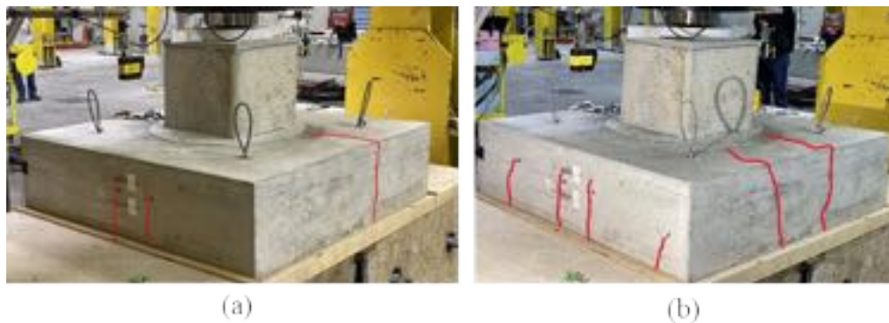
Figure B - 53: Rebar strain gages in the longitudinal reinforcement on bottom of Specimen SC-2 Cracking was first visually observed on all faces of SC-2 at the first stop at 175 kips, as shown in Figure B - 54 (a). A large crack formed from the bottom of the north face to the top face next to the plug. Existing cracks grew in size and length and additional cracks formed as the load was increased, see Figure B - 54 (b).
