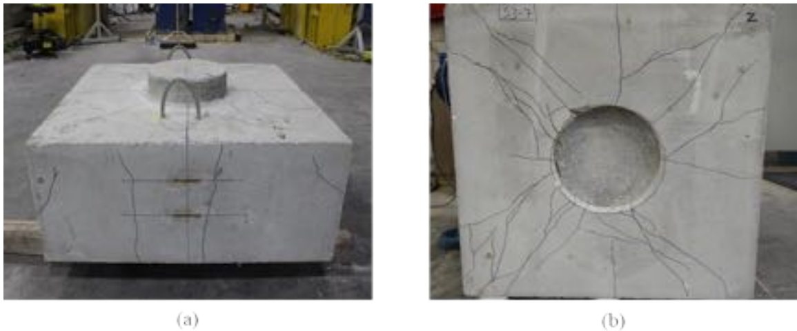
Figure A - 155: Cracking on (a) cap and (b) bottom of Specimen S3-7
