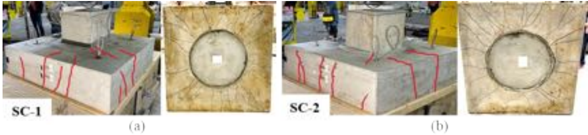
Figure 3-79: Cracking at failure for (a) SC-1 (sandblasted, 1/16-inch finish) and (b) SC-2 (metal pipe left in place)
