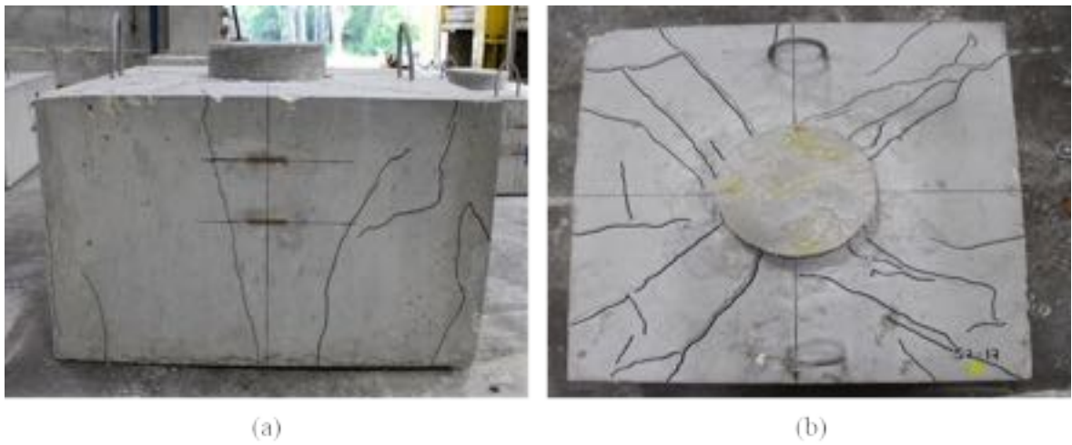
Figure A - 109: Cracking on the (a) east side and (b) top of the specimen S2-17
