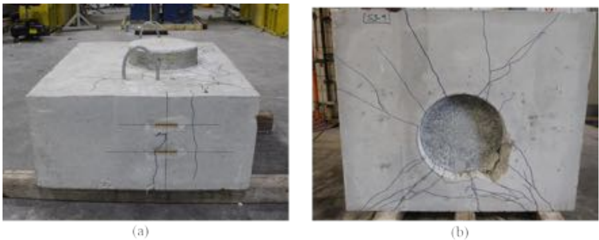
Figure A - 167: Cracking on (a) cap and (b) bottom of Specimen S3-9
