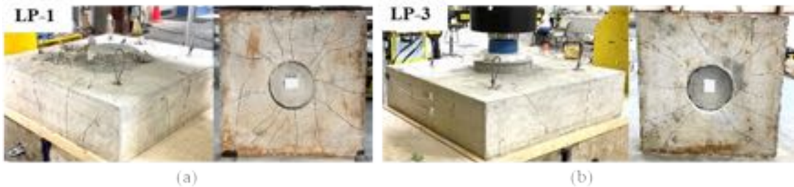
Figure 3-85: Crack patterns at failure for (a) LP-1 (smooth with 1/16-inch roughness) and (b) LP-3 (corrugated with 1/16-inch roughness)
