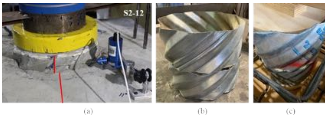
Figure 3-8: (a) Rotation observed in S2-12, (b) detail of the corrugated metal pipe when the pipe was left in place in later specimens, and (c) installed metal pipe with tape inside blocking voids
