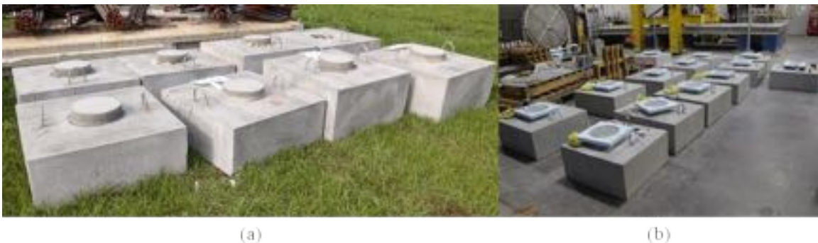
Figure 3-5: Finished specimens for (a) part of Series II and (b) Series III
