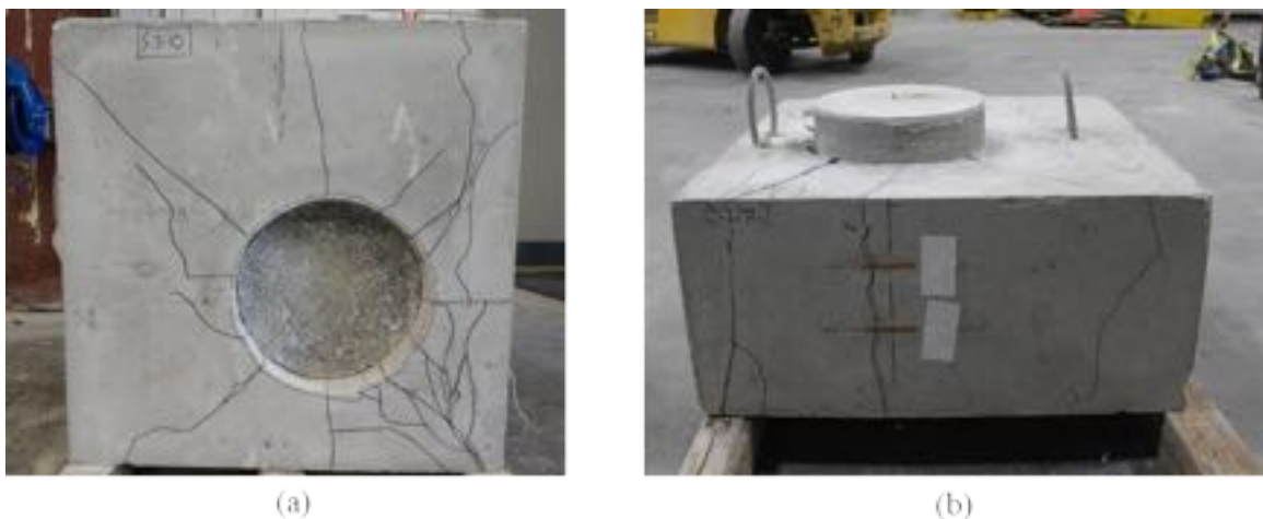
Figure A - 173: Cracking after testing on (a) bottom and (b) cap of Specimen S3-10
