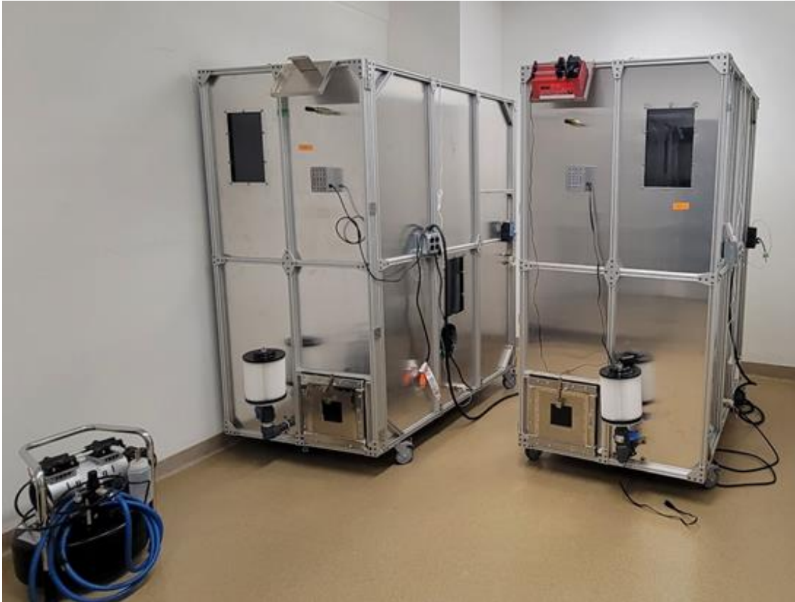
Figure 38. Whole-body aerosol exposure chambers used in the study were housed in the FIU animal care facility.
