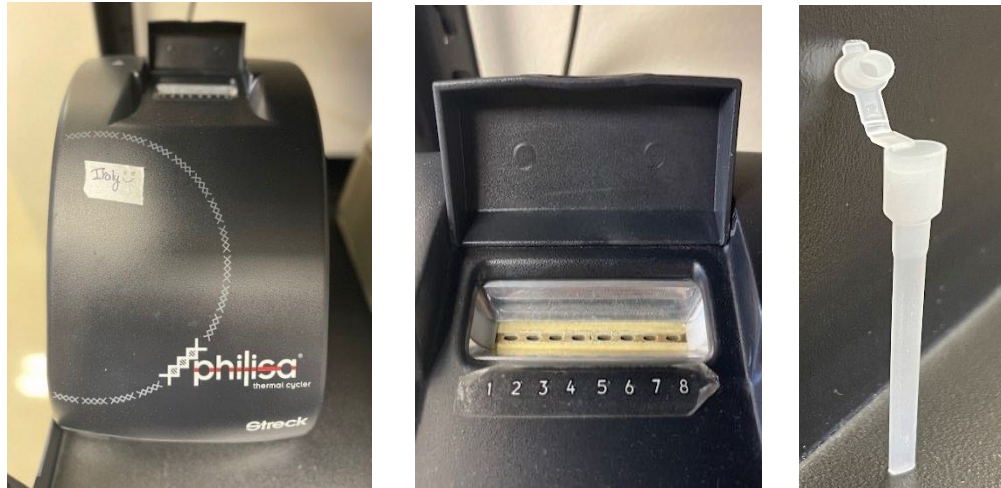
Fig. 35. Fast Thermal cycler Philisa ® from Streck Biosciences. Details of the heat block and the design of the tubes are shown.
