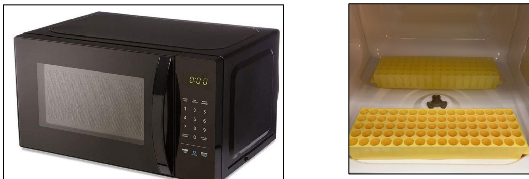
Fig.20 Commercial Microwave oven used for preliminary calibration tests (left), and sample racks registration inside the oven.
