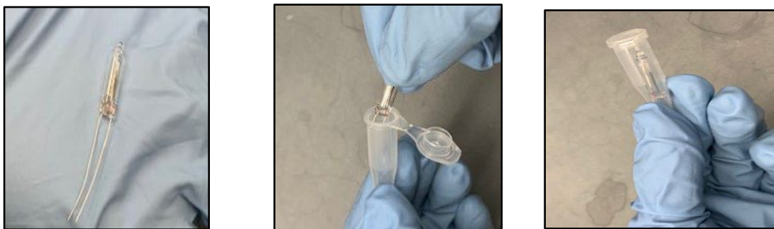
Fig.21 Neon bulbs set-up. First the electrodes were cut to fit the tube length, then they were carefully placed in the tube avoiding any contact between the filaments.
