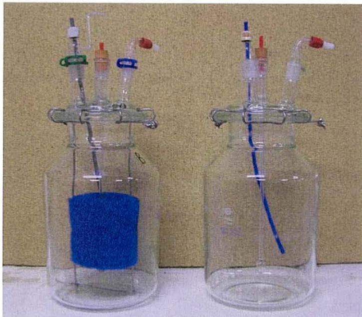
Figure 2.13 Single stage digesters with (left) and without (right) polyurethane foam biomass support media.
