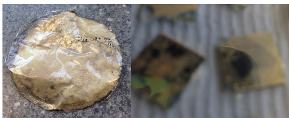
Figure 2.2 – Photographs showing the silver film supported on polystyrene (left) and 1.5 x 1.5 cm glass supports (right). Note the reflection shown by the silver on glass.
