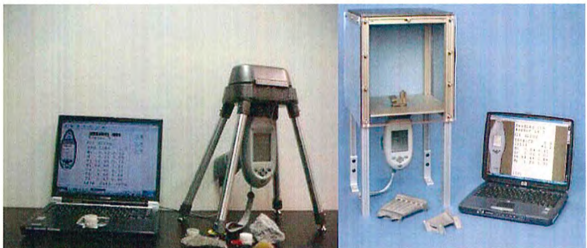
Figure 4-26. Niton XLP 300 Series shown with optional portable (part #500-961) and bench-top (part #600-705) test stands
