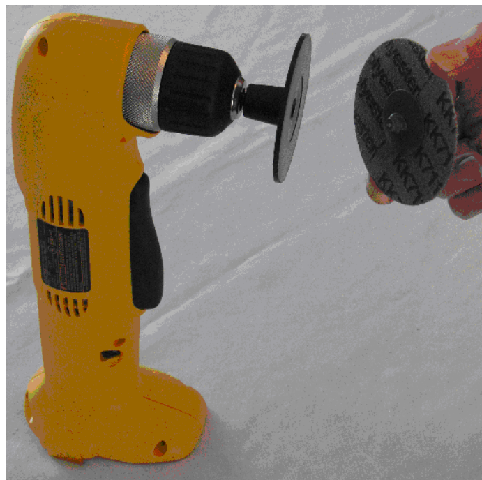
Figure 4. Attaching the Sanding Disc 2
