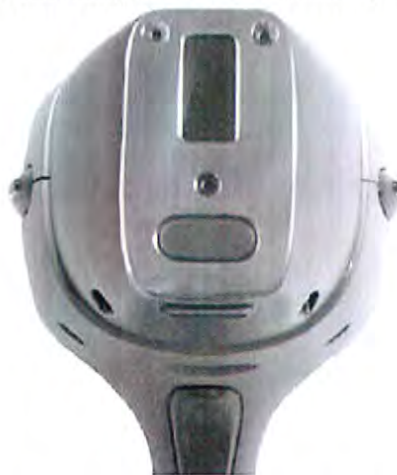
Figure 9-5. Fitting Face Plate over Proximity Button
