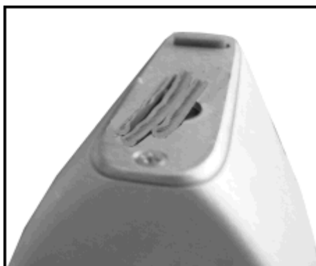
Figure 17. PVC Wire Insulation With Conductor Removed
