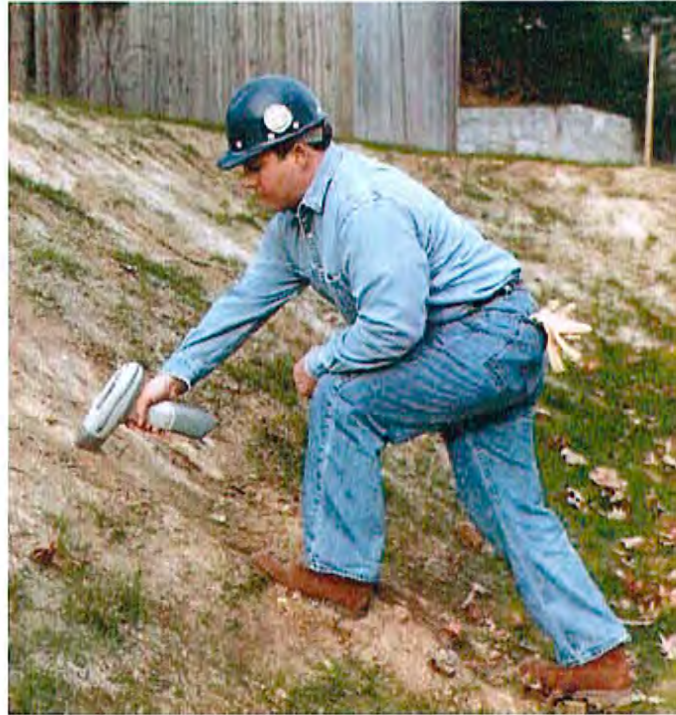
Figure 6-11. In-Situ Soil Testing
