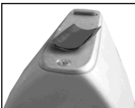
Figure 19. Correct Way to Measure Heat Shrink Tubing
