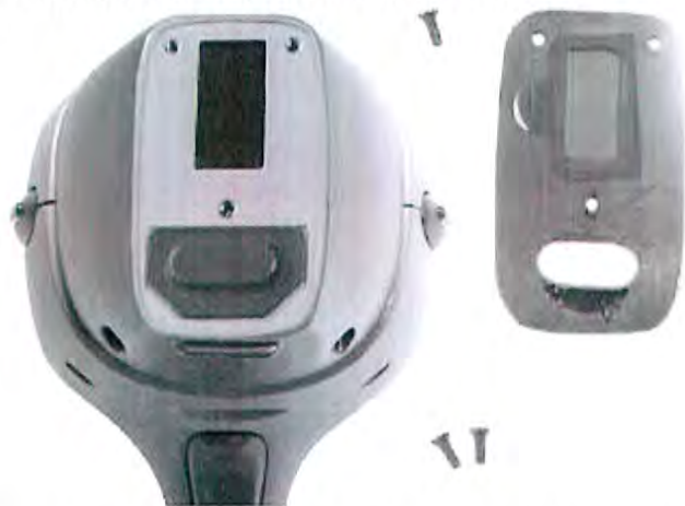
Figure 9-4. Face Plate Removed showing Kapton Window on Reverse
