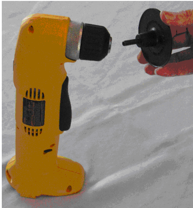
Figure 3. Attaching the Sanding Disc 1
