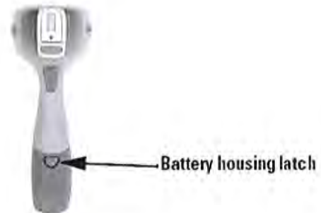
Figure 9-1. Location of the Battery Housing Latch
