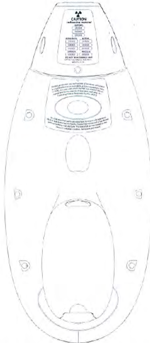
Figure 1-4. View of the Underside of the XLp Analyzer Showing Proper Placement of General and State Specific Radiation Labels
