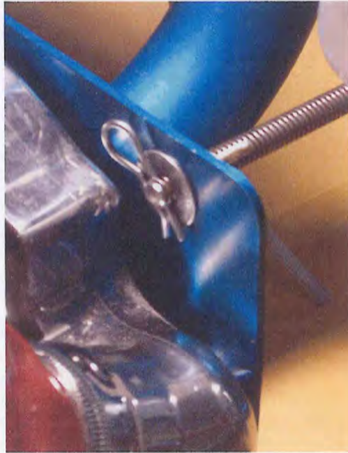
Adjusting screw with washer and clip mount to vacuum plate.
