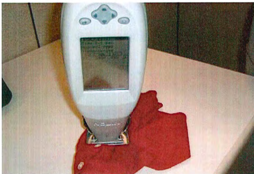
Figure 4-19. The sweater is placed on the table for measurement. Ensure the table has no lead by first measuring it with the analyzer.
