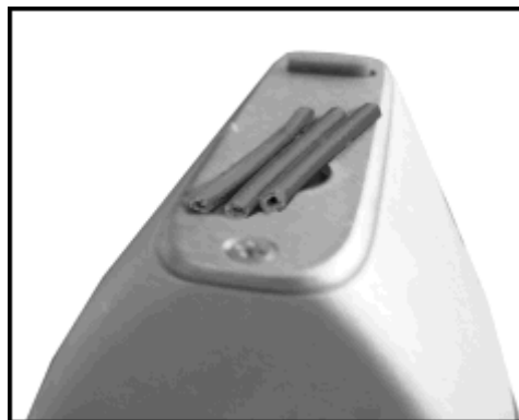
Figure 16. Wire Insulation Cut Into Strands
