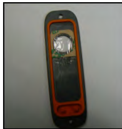
Figure 6. Measurement Window Replaced
