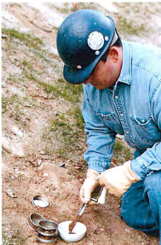
Figure 6-12. In-Situ Depth Profiling
