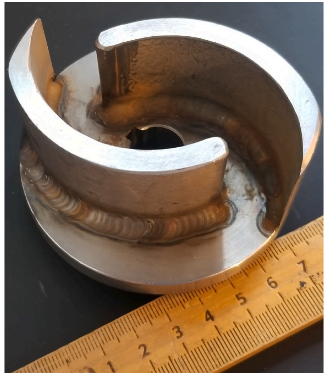
Fig. 4. MSTL pump impeller. The impeller is made of 316 stainless steel. The scale numbers are in cm.
