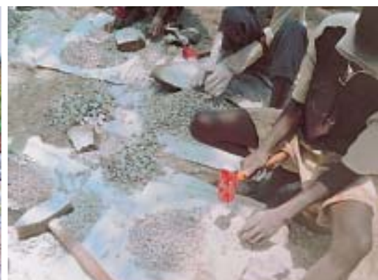
Dolomite crushing, Mkushi, Zambia.
