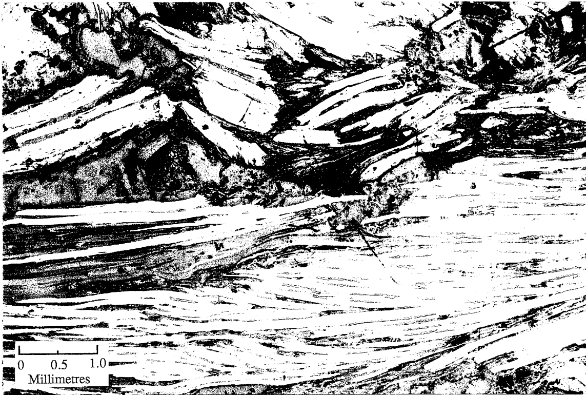
Figure 7. Photomicrograph of Njoka (B) graphite schist (reflected light)
