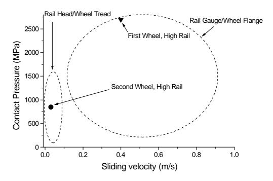
figure 9 Wheel/rail contact conditions on the Stockholm local railway network derived from GENSYS simulations [6] (also shown are results from Medyna simulations of the Älsvjö test track [16] for the first and second wheelsets)
