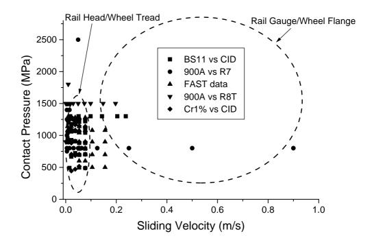
figure 11 Available rail steel wear data plotted over typical wheel/rail contact conditions
