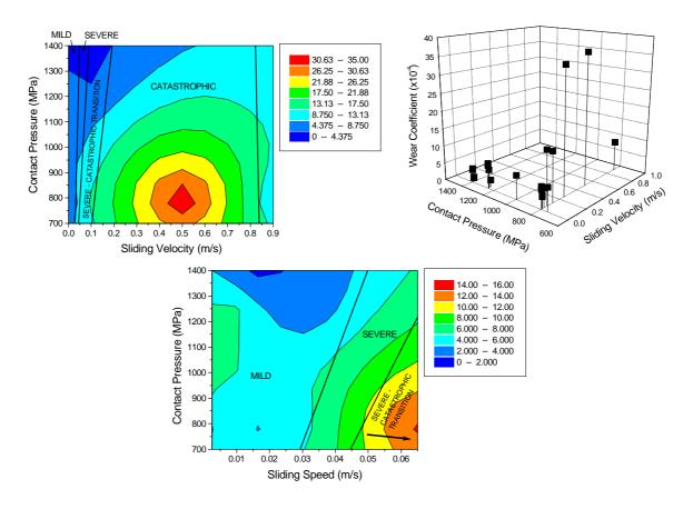
figure 7 Wear coefficient maps for UIC60 900A rail material versus R7 wheel material (data from [3])
