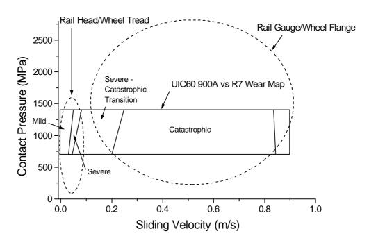
figure 10 UIC60 900A rail steel wear map plotted over wheel/rail contact conditions derived from GENSYS simulations [6]
