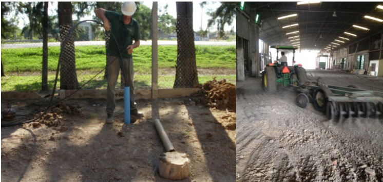
Pictures 7 and 8. Invasive soil and water table sampling tasks in a property contaminated with agrochemicals (Villa Ocampo, Argentina)
