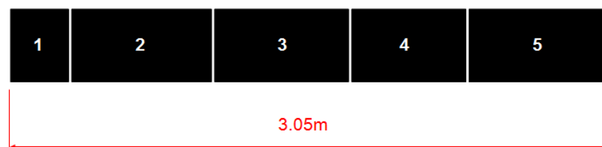
Figure 2. Characteristics of an artificial coal seam for sorption testing. The lengths of coal blocks 1 to 5 are 0.31 m, 0.74 m, 0.70 m, 0.60 m, and 0.70 m, respectively.
