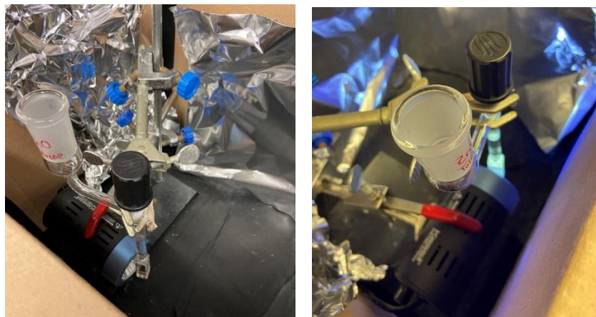
Figure 5.32 (left) UV irradiation setup in dark cardboard box lined with aluminum foil and Kontes cuvette with sample held ~1 cm from lamp. (right) Upon turning the lamp on, visible emission of the ZnO nanocrystals is evident, indicating successful excitation with irradiation.
