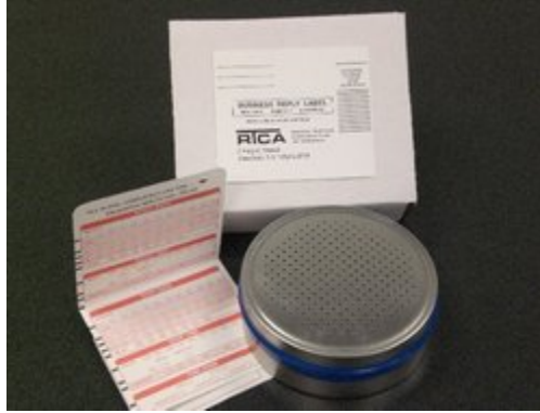
Figure 1: Charcoal canister from Radon Testing Corporation of America, similar to those used in the State Residential Radon Survey
