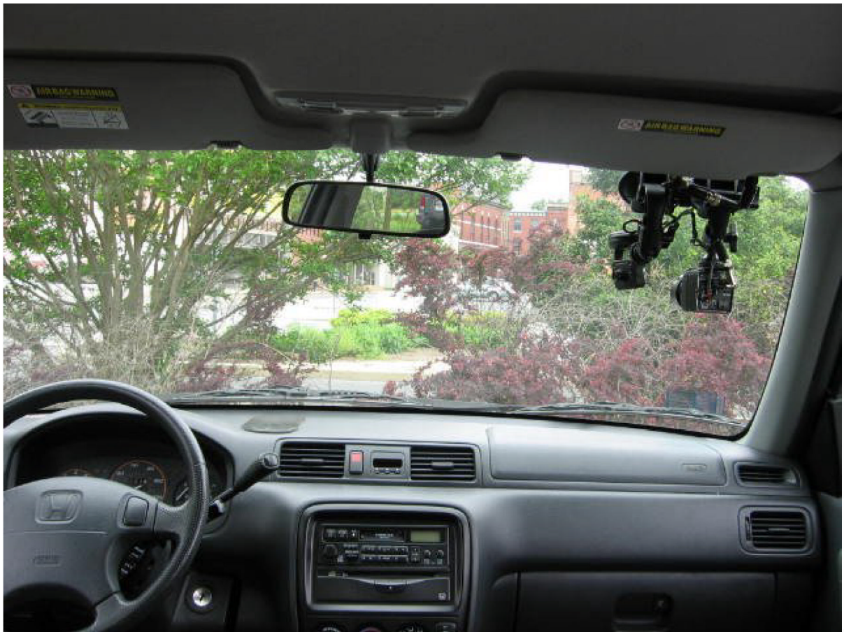
Figure 1. Driving monitoring system installed in a vehicle. Image shows the forward facing color camera which captures footage on the road and the monochrome camera capturing the driver both mounted on the passenger side of the vehicle
