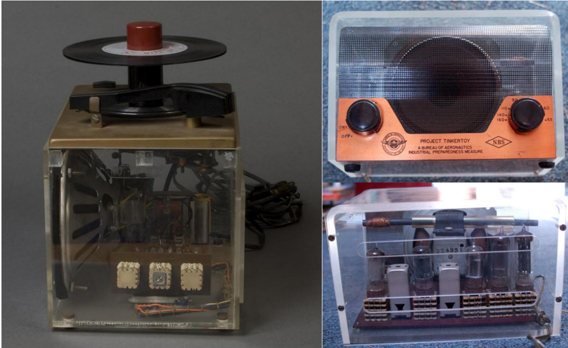
Figure 7. Portable record player (left), front of radio (top-right), and back of radio (bottom-right) made with a clear case to display the modular electronics developed in Project Tinkertory. National Institute of Standards and Technology, U.S. Department of Commerce, image #17431, https://www.nist.gov/image-17431 , accessed 28 September 2022.
