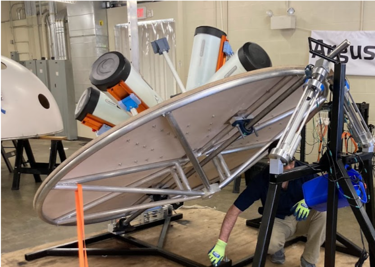
Figure 6.2 Telescope support platform, installed on the low-cost “Hercules” mount structure, during lab integration testing.
