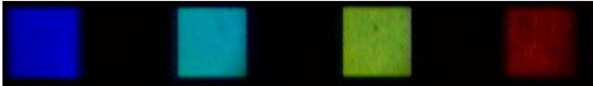
Figure 10. Confocal microscope image of nc-VO 2 arrays ordered by increasing interparticle spacing from left to right.
