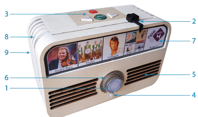
Figure 3. High-fidelity prototype of the music player, with the following components: 1. Volume knob, 2. Presets slider, 3. Control buttons (start, stop, previous, next), 4. Motion sensor, 5. Speakers, 6. Volume indicator, 7. Presets, images with light, 8. Product light, 9. Ambient light (on the back).
