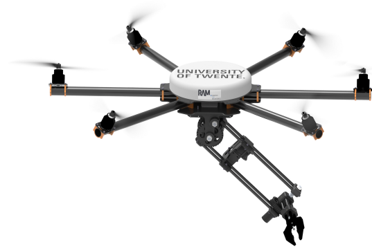
Fig. 1: Example of AM: the aerial manipulator at RAM-UT, with a fully actuated hexarotor aerial vehicle and a 3-DoF arm, thus 9-DoFs in total.
