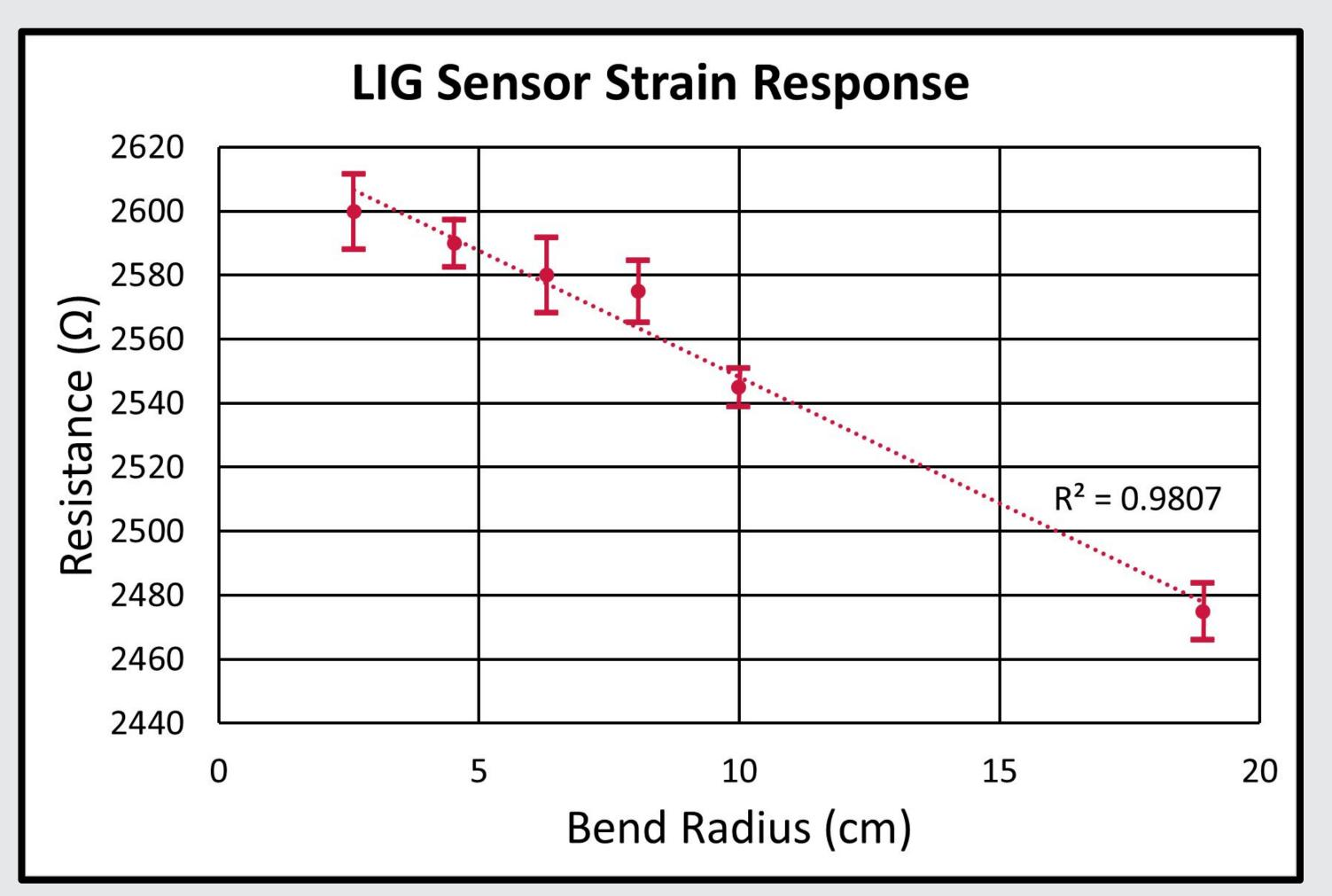
The resistance of the trace appears to decrease linearly with increasing bend radius, compared to a baseline of  $2450\pm9.60 \Omega$ . Error bars indicate one standard deviation.
