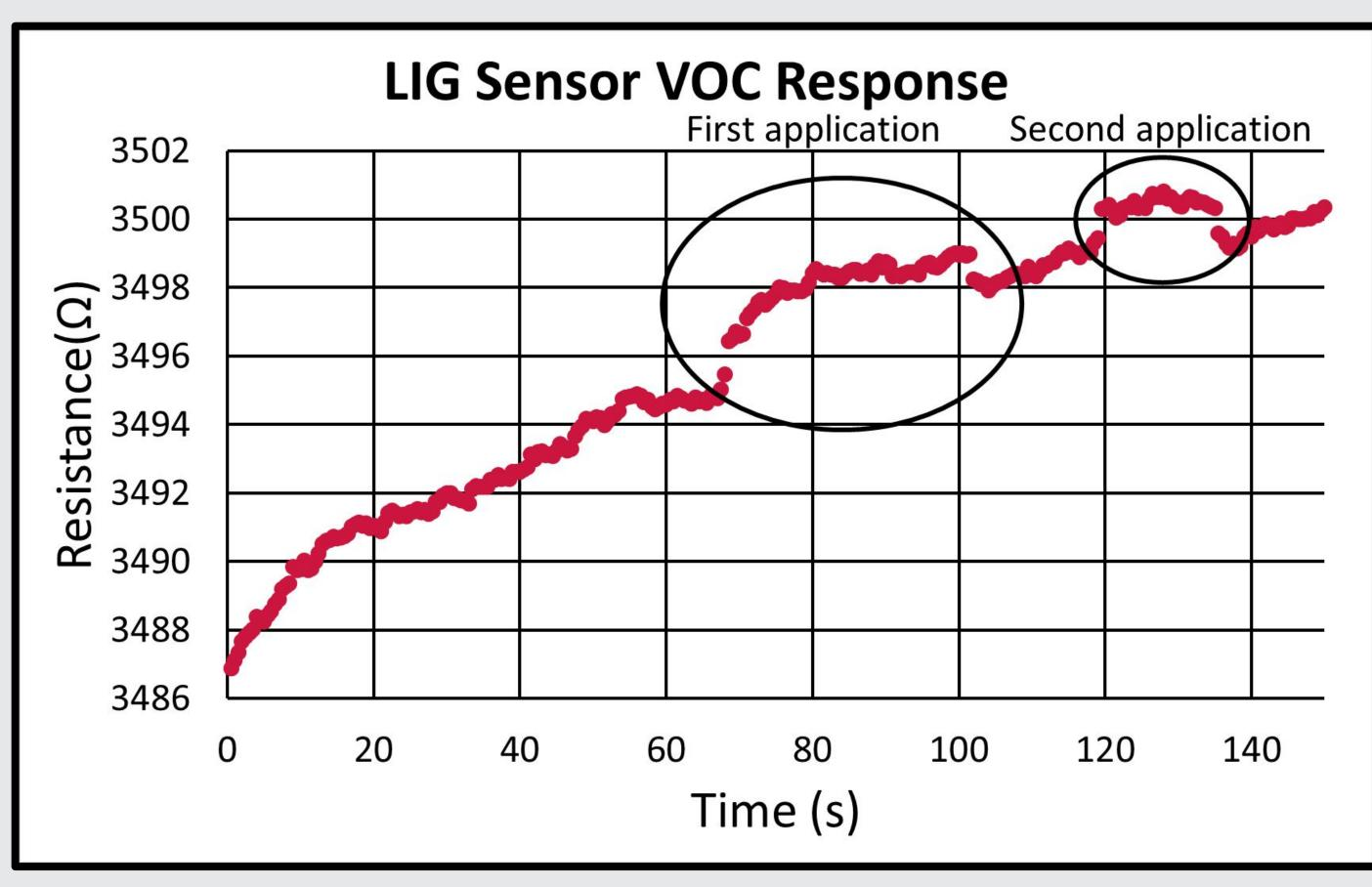
During a typical recording session, a syringe of concentrated VOCs is depressed above the sensor's surface. There will be a small increase in resistance for several seconds, before it decreases again. This concentration was procured using Wyoming Big Sagebrush leaves.
