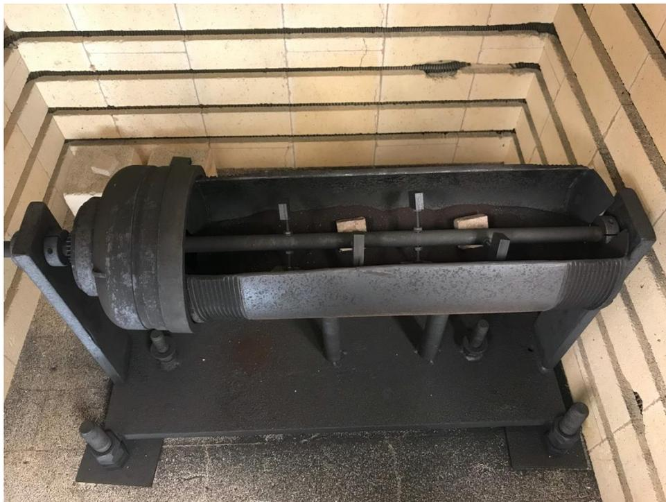
Figure 3: Abrasion test setup for testing at 800 °C. Mounted in this image are SS316, Inconel 740H, and fireclay cement type refractory specimens running through a bed of HSP 40/70 particles.
