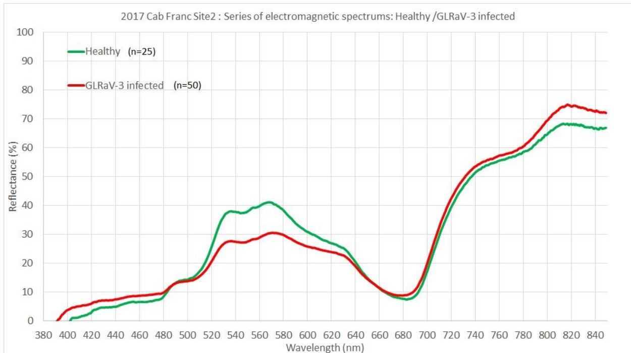
Figure 6.2. The series of electromagnetic spectra from healthy and GLRaV-3 infected Cabernet franc leaves measured by hand-held spectrometer at site 2.
