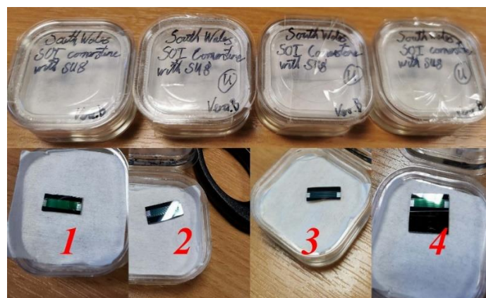
Figure 5.1 Photos of the first batch of SOI chips (with SU-8 covered taper coupler), from left to right is the chips No. 1,2,3, and 4, respectively
