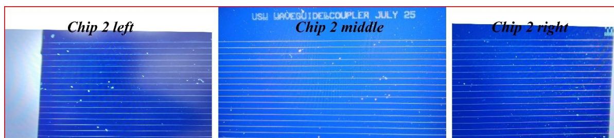
Figure A 4 Microscope view of SOI waveguide with free space taper coupler No.2
