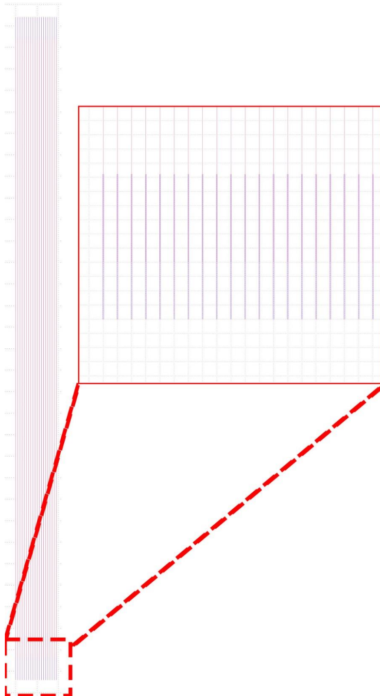
Figure A 1 Mask of a group of SOI waveguides with SU-8 cladding coupler at both ends.
