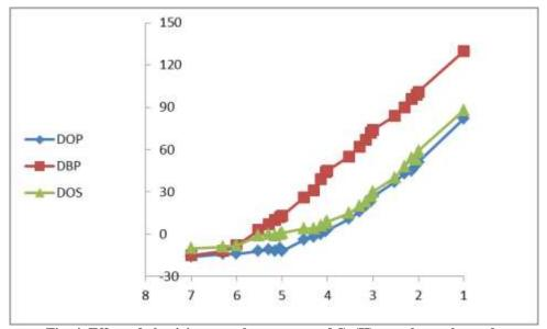
Fig. 4. Effect of plasticizers on the response of Cu(II)-membran electrode (32% PVC, 64% plasticizer, 3% complex as ionophor, 3% NaTPB as addative).
