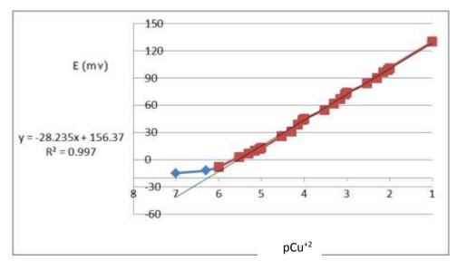
Fig. (2): calibration curve of Cu(II)-membrane electrode (No 14).
