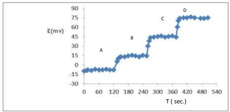
Fig.( 6). Potential–time plot for the response of Cu(II)-membrane electrode electrode (32% PVC , 64%DBP , 3% complex as ionophor, 3% NaTPB as addative) for step changes in concentrateion of Cu(II): (A)  $1.0x10^{-6}$  M, (B)  $1.0x10^{-5}$  M, (C)  $1.0x10^{-4}$  M, (D)  $1.0x10^{-3}$  M.
