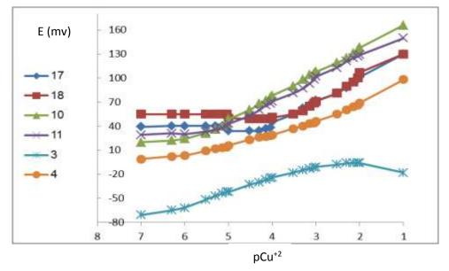
**Fig. (3): Potential response of Cu(II)-membrane electrodes (3,4,10,11,17,18) of different composition.**
