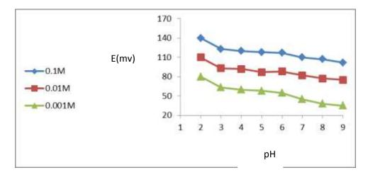
Fig. 5. Effect of pH of test Cu(NO<sub>3</sub>)<sub>2</sub> solution on Cu(II)-membran electrode (32% PVC, 64%DBP, 3% complex as ionophor, 3% NaTPB as addative).
