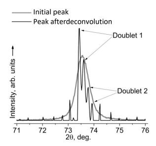
Fig. 6. The initial peak (220) and peak after deconvolution on the diffraction pattern of the Cu–3Pd–3Ag alloy, cryodeformation ( $e\approx3.5$ ) + 250 °C, 1 h, cooling in water
