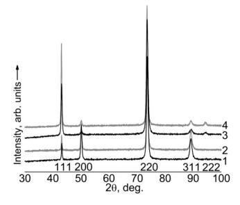
**Fig. 5.** Diffraction patterns of the Cu–3Pd–3Ag alloy specimens:  $1 - deformation at room temperature (e<math>\approx$ 3.5); 2 - treatment (1) + 250 °C, 1 h, cooling in water;  $3 - cryodeformation (e \approx 3.5); 4 - treatment (3) + 250 °C$ , 1 h, cooling in water
