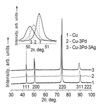
Fig. 1. Diffraction patterns of copper (1), Cu-3Pd (2) and Cu-3Pd-3Ag (3) alloys after cryodeformation (e $\approx$ 3.5)
