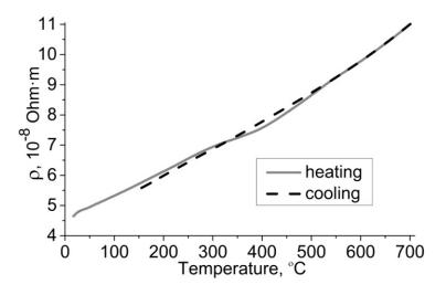
*Fig. 3.* Change in electrical resistivity at heating and cooling at a rate of 120 deg./h of the Cu–3Pd–3Ag alloy specimen drawing-deformed at room temperature ( $\approx$ 7.1)
