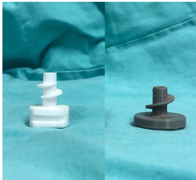
Figure 3. Comparison of the screw mechanism of the prototype (gray) and the model device (white).
