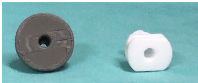
Figure 5. Comparison of the base of the old device (white) and the prototype (gray).
