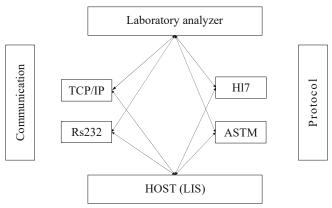
Fig. 2. The interaction model with the laboratory analyzer
