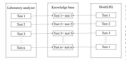
Fig. 3. Knowledge base of relationships between the analyzer and the laboratory information system
