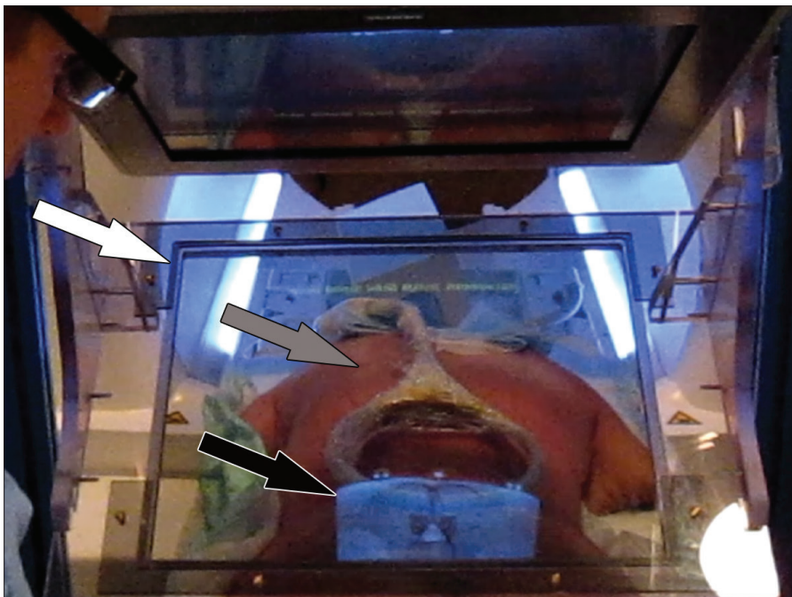
Figure 2. Procedural photograph demonstrating the operator's augmented reality consisting of a hybrid view of MR image and underlying cadaver. The hybrid view is being created by the reflection of the target MR image (black arrow) from a semitransparent mirror (white arrow) into the line of sight of the operator, where it merges with the underlying cadaver (gray arrow). Location, size, and skin contour of MR image and cadaver are matched through co-registration by the image-overlay navigation system.
